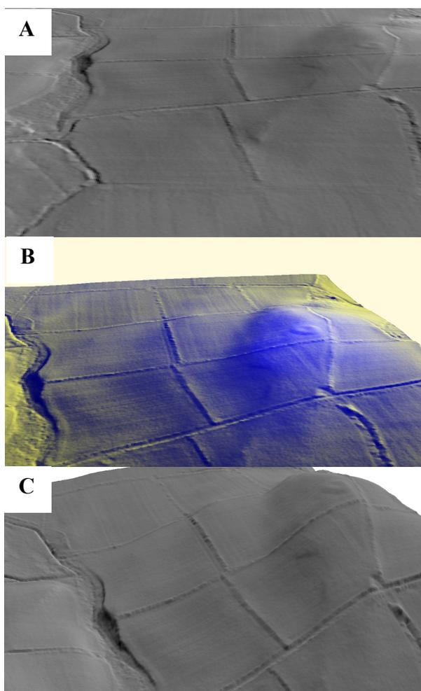
Figure 17 | Hillshade of Cross Oak Hillfort show draped across the LiDAR DTM facing north. Vertical exaggeration has been modified for each image: A-1x, B- 2x, C-5x. The Colouring in image B corresponds to band variation in the Hillshade, denoting the blue as higher elevation.
